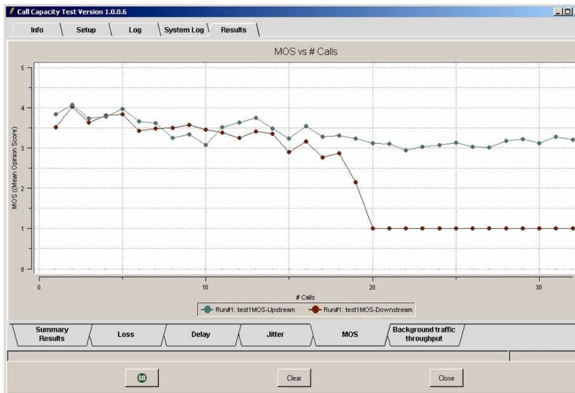
Figure 4: The Call Capacity test increments the number of calls going through the infrastructure in a controlled way. It measures and plots delay, jitter and frame loss on each active call and then computes the R-Factor and MOS voice quality metrics for each call.
